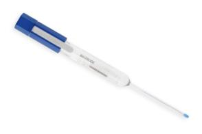
Commonly used for microtiter plate applications (especially solutions containing protein), a slim tip allows for immersion depth of only 7 mm.
