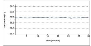
The incubation chamber's temperature stability of  $\pm 0.1^{\circ}$ C ensures experiment stability.
