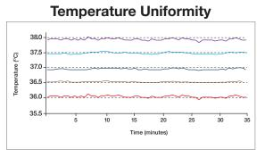
The incubated shaker's chamber's temperature uniformity  $(\leq \pm 1.5^{\circ}C)$  enables all samples to be heated evenly.
