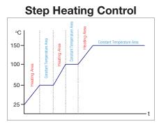
In program control mode, the controller allows the operator to set up step heating control.
