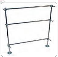
Setup with foot plates secured to a bench. Two-dimensional lattices can be assembled in units of  $24'' \times 24''$  with the crossbars horizontal or vertical. The set allows construction of up to two  $24'' \times 24''$  sections with one crossbar each.
