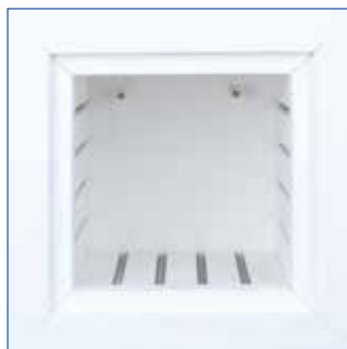
Inner Chamber of Exposed Heating Elements-type
