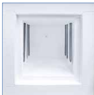
Inner Chamber of Exposed Heating Elements-type
