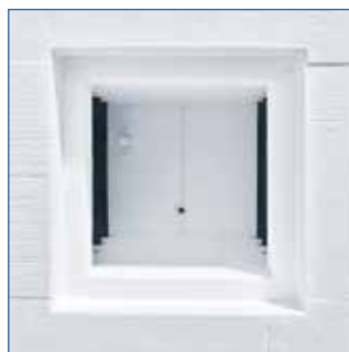
Inner Chamber of Exposed Heating Elements-type
