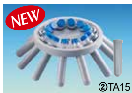
②TA15 (2) Fixed Angle Rotor ; 10~15ml 15Holes, “R1512”
