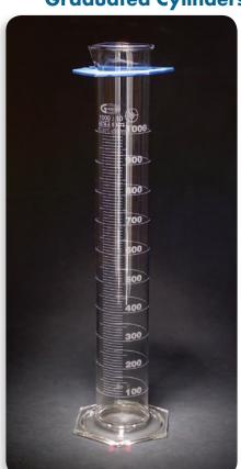
Cylinders comply with ASTM E1272, Class A, meets USP standards, individually serialized and certified.
