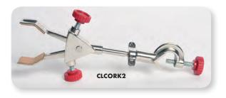
Our deluxe line of 2-prong burette clamps are made of pressure die-cast zinc alloy and are chrome plated. Adjustable to hold up to 60mm O.D. burettes, these clamps feature a spring-type adjustment key. Boss head clamp can swing freely and is lockable at any angle up to 360°, and can be used with rods up to 19mm.
