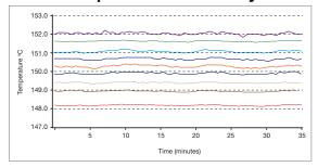
The drying chamber's temperature uniformity enables all samples to be heated evenly.
