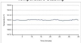
The drying chamber's temperature stability of  $\pm 0.5^{\circ}\text{C}$  ensures experiment stability.
