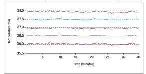
The incubation chamber's temperature uniformity enables all samples to be heated evenly.
