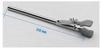
**CLAMP FOR BURETTES AND TUBES** Made of chrome plated metal with two prong jaws coated with PVC. For Ø from 7 to 25 mm. Part No. 7000130
