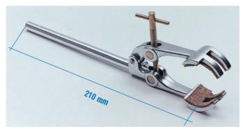
UNIVERSAL CLAMP "MINIMAX" Made of Dur-aluminium with cork lined jaws. For Ø from 0 to 80 mm. Part No. 7000403
