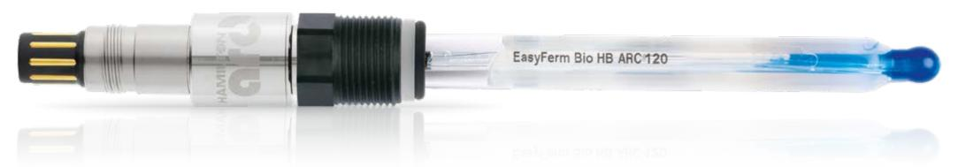
**Specifications** Measuring range 0 to 14 pH Process temperature 0 to 140 °C (Arc: analog 0 to 110 °C, digital 0 to 140 °C) 0 to 6 bar Pressure range (relative to ambient) Hygienic aspects Autoclavable, SIP, CIP HB, PHI pH glass Electrolyte Foodlyte Everef-F Reference system Diaphragm **HP** Coatramic O-ring Silicone
