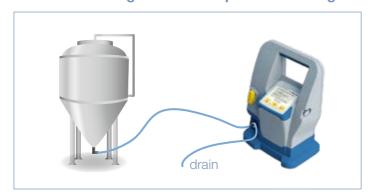
Beverly can be used as shown in the pictures and even beyond. An additional application is to check the oxygen content of the exhaust gas of vessels while flushing with CO<sub>2</sub> after cleaning and prior to filling. Measuring the oxygen at this point can help to save time and CO<sub>2</sub>. Even if Beverly stays connected to a pipe or a vessel while CIP is running it's robust stainless steel flow cell prevents damage.
