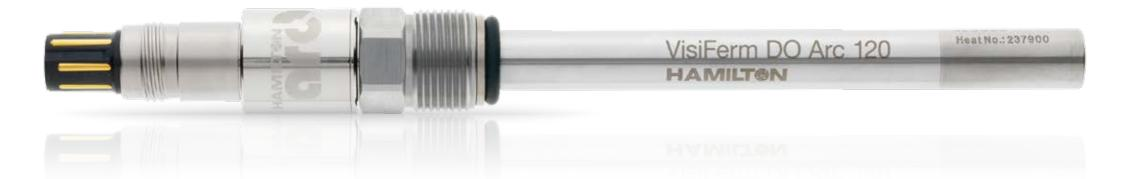
The VisiFerm DO is the first optical oxygen sensor with integrated opto-electronics, having the full functionality of a measuring device with self-diagnostics. It is steam sterilizable, autoclavable and CIP compatible. The VisiFerm requires less maintenance than a classical oxygen sensor as it does not have a mechanically sensitive membrane or a corrosive electrolyte.
