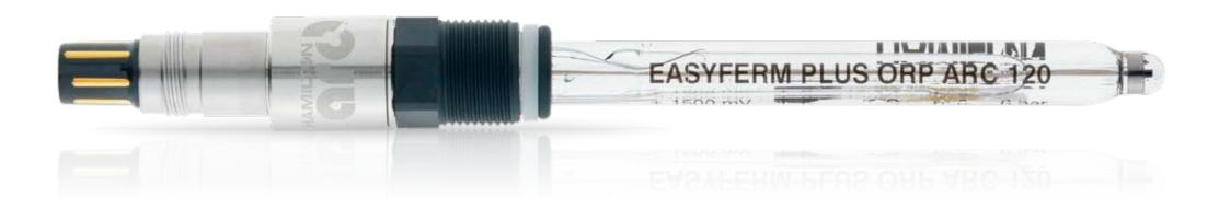
**Specifications** Measuring range ± 2000 mV (Arc: ± 1500 mV) Process temperature 0 to 140 °C (Arc: analog 0 to 110 °C, digital 0 to 140 °C) Pressure range 0 to 6 bar (relative to ambient) Hygienic aspects Autoclavable, CIP, SIP ORP element Pt ring Electrolyte Phermlyte Everef-F Reference system Diaphragm **HP** Coatramic O-ring **EPDM**
