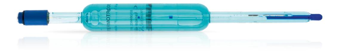
The maintenance free FermoTrode sensors are designed for measuring pH in pharmaceutical and biotechnological industries and fit in the MasterFit and RetractoMaster housings. The Everef-F reference cartridge ensures that the reference electrolyte Skylyte remains free of silver and precipitation, and withstands steam sterilization.
