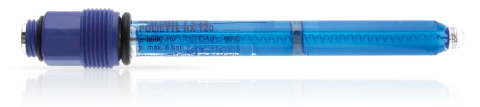
**Specifications** ± 2000 mV Measuring range Process temperature Polilyte Pro: -10 to 60 °C Polyplast Pro: -10 to 40 °C 0 to 6 bar Pressure range (relative to ambient) ORP element Pt-wire Polisolve Electrolyte Reference system Polilyte Pro: Everef-B Polyplast Pro: Ag/AgCl Diaphragm Single Pore O-ring Polilyte RX: EPDM Polyplast Pro RX: EPDM
