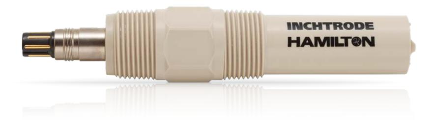
**Specifications** Measuring range 0 to 14 pH Process temperature -10 to 130 °C (flat membrane) 0 to 130 °C (cylindrical membrane) 0 to 10 bar (25 °C) Pressure range (relative to ambient) 0 to 6 bar (130 °C) pH glass HF (flat membrane) PHI (cylindrical membrane) Electrolyte Polisolve Reference system Everef-L Diaphragm Single Pore Temperature sensor Pt1000 in VP version Pt100 in fix cable version
