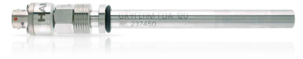
The OxyFerm FDA is an electrochemical oxygen sensor suited for applications with high demands for hygiene, e.g. in pharmaceutical industry, in biotechnology and in food & beverage production. It is available with 12 mm or 25 mm (XL) shaft diameter.
