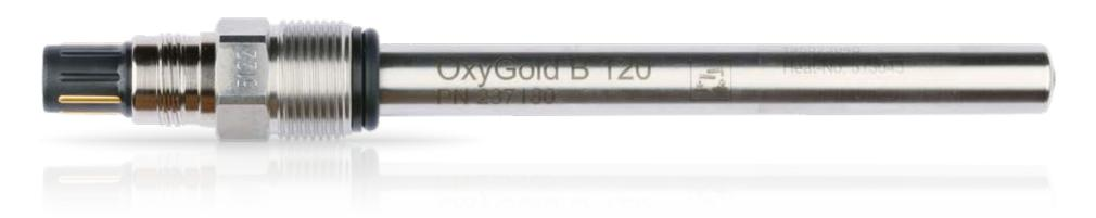
**Specifications** 8 ppb to 40 ppm (DO) Measuring range Response time t98% < 60 s at 25 °C, from air to nitrogen 0 to 100 °C Process temperature Pressure range 0 to 12 bar (relative to ambient) CIP Hygienic aspects Oxylyte B Electrolyte Surface Quality  $R_a < 0.4 \mu m (N5)$ Current in air at 25°C 180 to 500 nA Material Stainless steel 1.4435 Polarization voltage 0 mV **EPDM** O-ring
