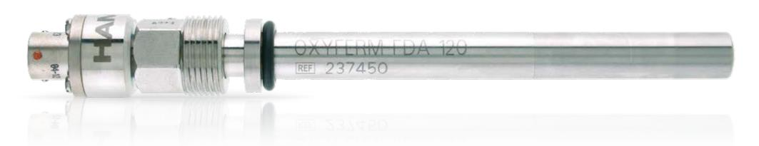
10 ppb to 40 ppm (DO) Measuring range Response time t98% < 60 s at 25 °C, from air to nitrogen 0 to 130 °C (Arc: analog 0 to 110 °C, Process temperature digital 0 to 130 °C) Pressure range 0 to 4 bar (relative to ambient) Autoclavable, CIP, SIP Hygienic aspects Electrolyte Oxylyte Surface Quality  $R_a < 0.4 \mu m (N5)$ Current in air at 25°C 40 to 80 nA Material Stainless steel 1.4435 -670 mV Polarization voltage **EPDM** O-ring
