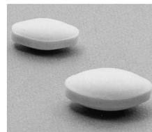
**Oval stir bar**, coated with PTFE, resistant to high temperatures of up to +275 °C. Can be used for all types, including
